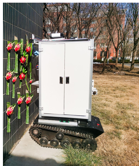
Figure 15. Physical prototype drawing of a picking and selecting integrated remote-operation-type dragon-fruit-picking device.
